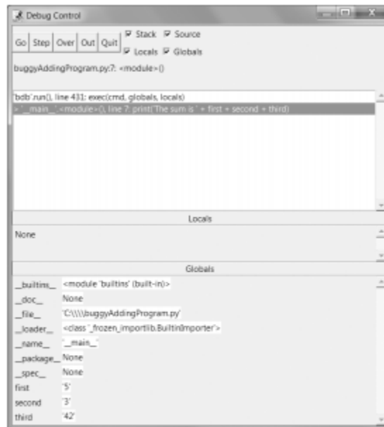
Figure 10-4: The Debug Control window on the last line. The variables are set to strings, causing the bug.
