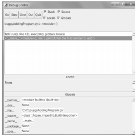
Figure 10-2: The Debug Control window when the program first starts under the debugger
